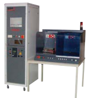
Electrical safety tester for safety test Automatic test system DTS-ST for electrical safety test of instruments, appliances and assemblies
